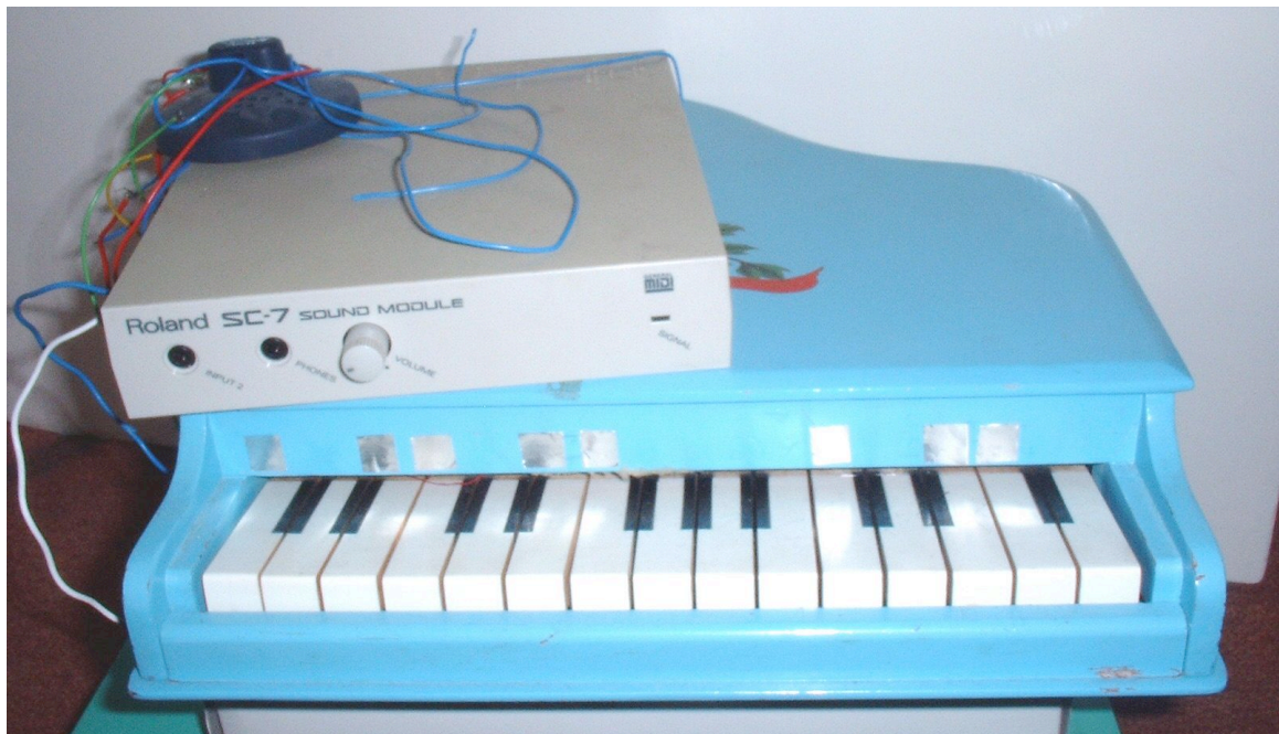
Figure 4 – Hybrid toy piano and MIDI Sound Module.
