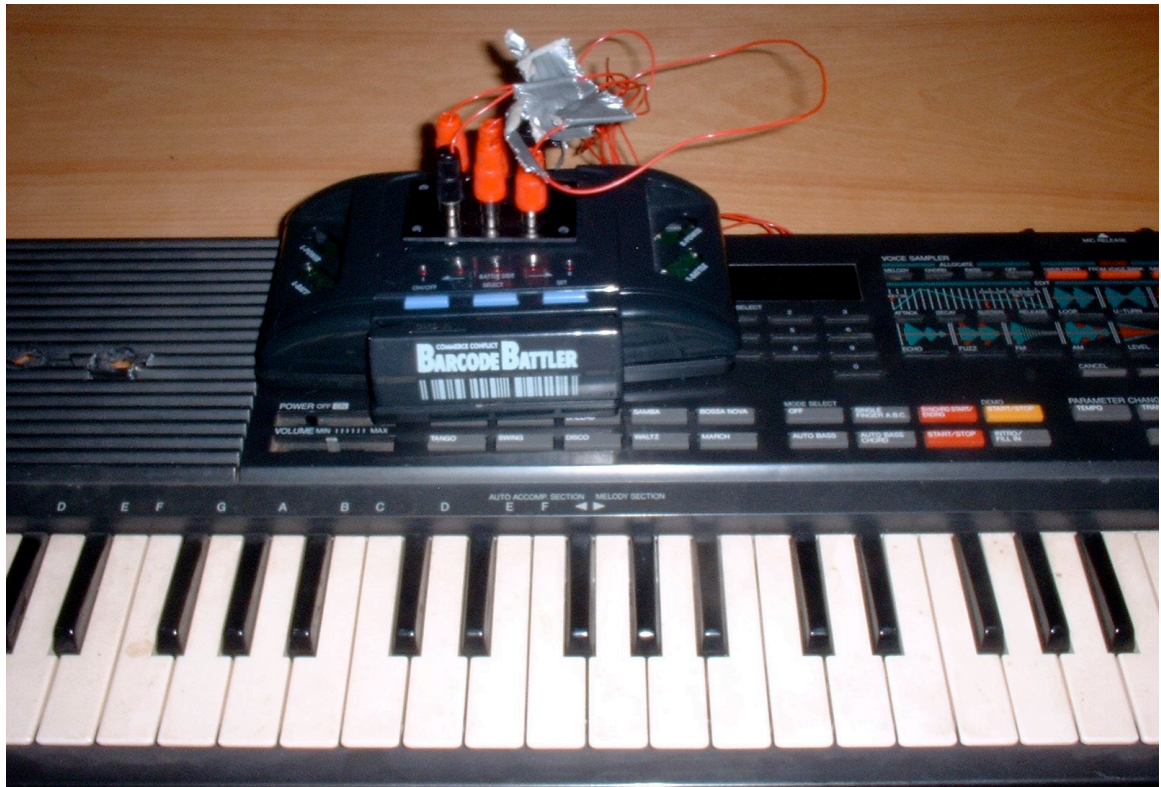
Figure 5 - Hybrid 'Barcode Battler' and Yamaha VSS-220 keyboard.
